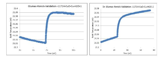
Figure 5: Calorimeter traces from reactive tests (Al crucible, CuO, Cu, H<sub>2</sub>O).
