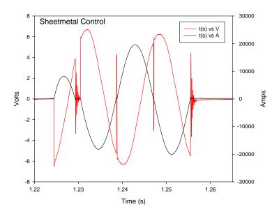
Figure 1: Nickel sheet control on the instrumented spot welder.
