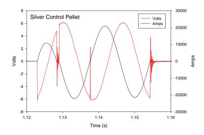
Figure 2: Traces from the test using a silver control pellet.
