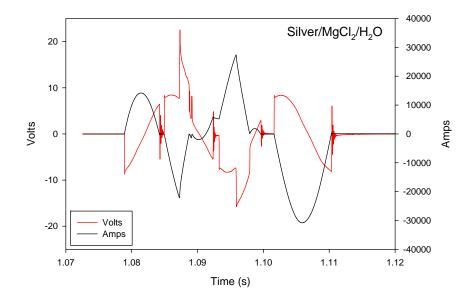
*Figure 3: The current and voltage traces for Test 8 (Silver/MgCl<sub>2</sub>/H<sub>2</sub>O). Integrated power was 1582 Joules.*
