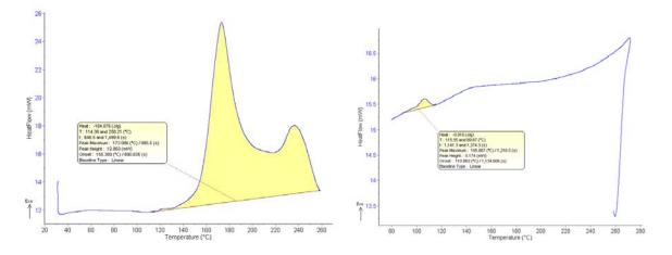
*Figure 6: Heating (left) and cooling (right) traces for the reactive test sample.*
