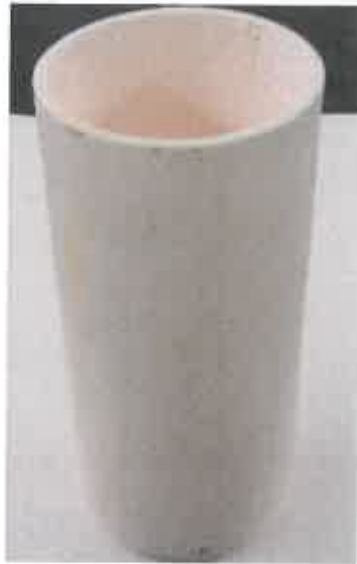
Figure 6. Ceramic Cylindrical Crucible Cell Container.
