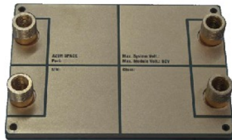
Back of Dense Receiver Array With Cooling Water Inlets and Outlets
