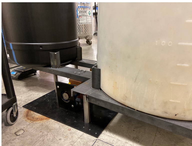
Figure 2. Image showing weighing system composed of cantilever with (from left to right) scale, counterweight, and water-bath tank for submerged cell.
