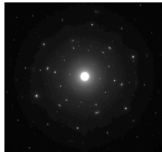
GaOOH:H 2 (1/4) SAED Orthorhombic Pattern
