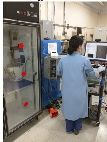
Fig. 1 – The setup of the Parr 1341 calorimeter used for the energy balance determination.
