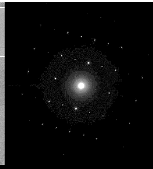
GaOOH:H 2 (1/4) SAED Orthorhombic Pattern
