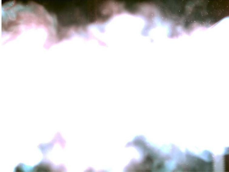
Figure 2: Supersonic expanding plasma formed from the high-current detonation of the solid fuel  $\text{Cu} + \text{CuO} + \text{H}_2\text{O}$  filmed at 6500 frames per second.
