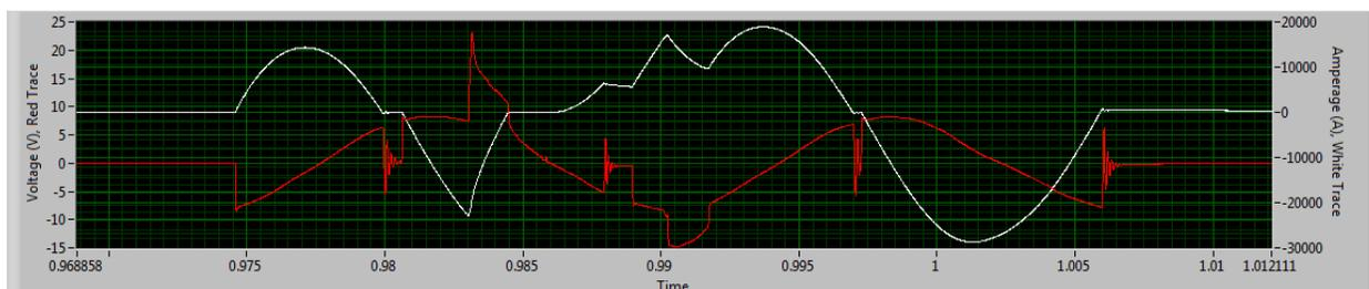
Figure 4: The current and voltage traces for Test 7 (Silver/MgCl<sub>2</sub>/H<sub>2</sub>O).
