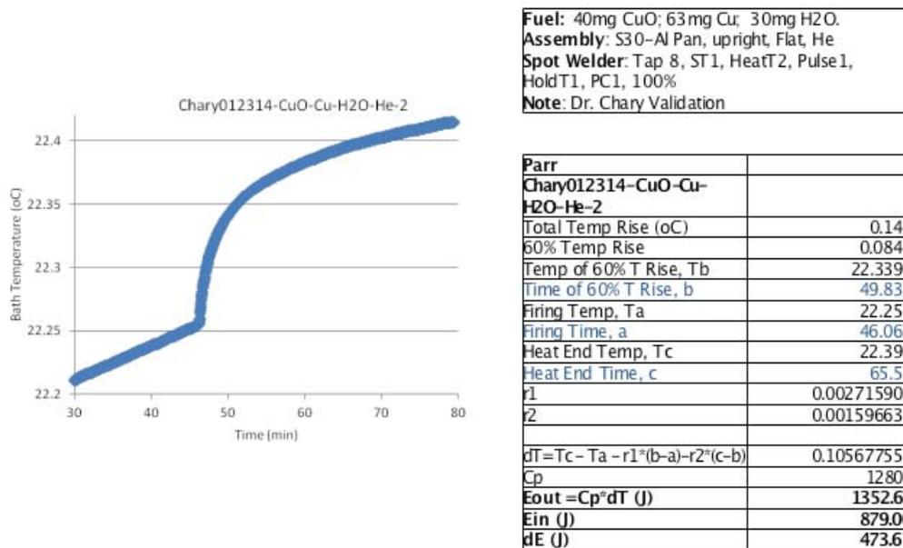
Figure 8. Second validation test of solid fuel  $CuO + Cu + H_2O$ .
