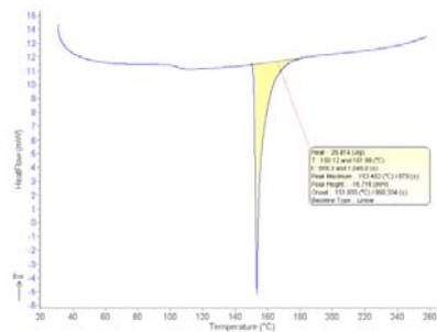
Figure 10. Indium metal, DSC heating trace.
