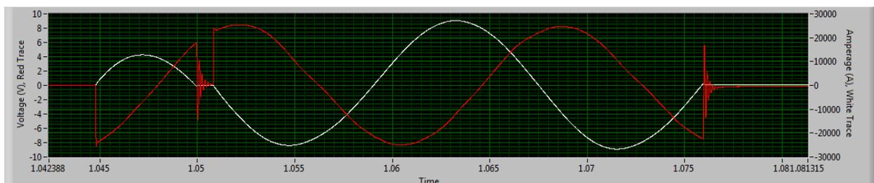
Figure 1: Nickel sheet control on the instrumented spot welder.
