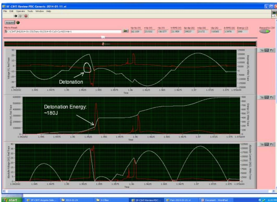
Figure 5. The voltage and current (top), power and energy (middle), and absolute voltage and absolute current (bottom). The detonation is indicated by the disruption of the waveform. The detonation occurs at 180 J input energy, about 20% of the total input energy.
