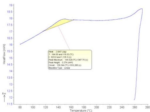
Figure 13.  $\text{Cu}(\text{OH})_2 + \text{FeBr}_2$ , DSC cooling trace.
