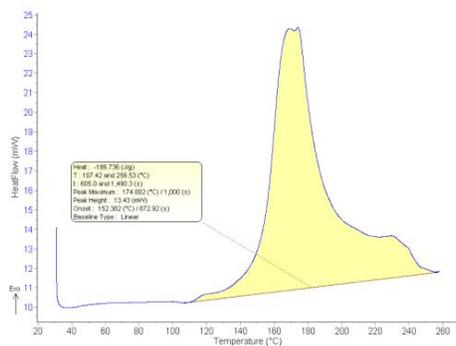
Figure 12.  $\text{Cu}(\text{OH})_2 + \text{FeBr}_2$ , DSC heating trace.
