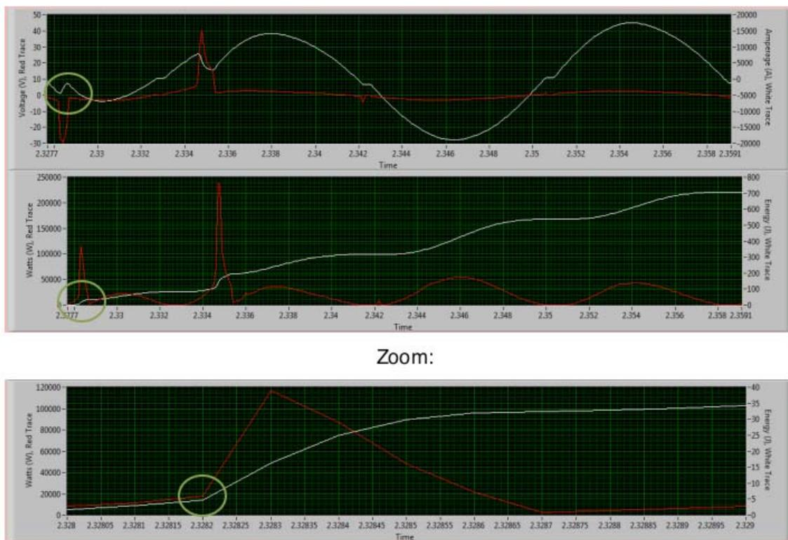
Figure 7. The voltage and current (top), power and energy (middle), and expansion of the power and energy traces (bottom). The detonation is indicated by the disruption of the waveform. The detonation occurs at 5 J input energy, less than 1% of the total input energy and 1% of the output energy.
