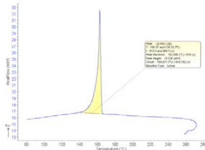
Figure 11. Indium metal, DSC cooling trace.
